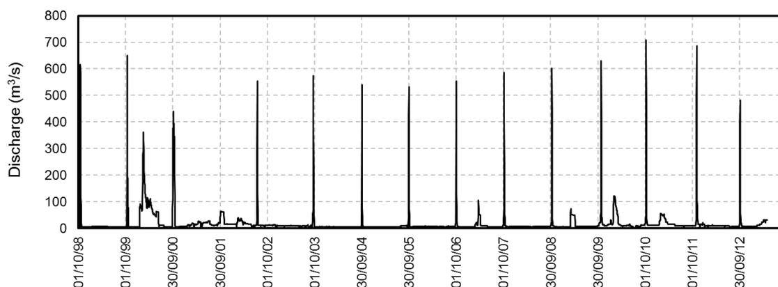
**Figure 9.4** Plot of releases from Jozini Dam into the Pongola River gauged at Station W4H013 (refer to Figure 9.3), for the period 1998 to 2012
