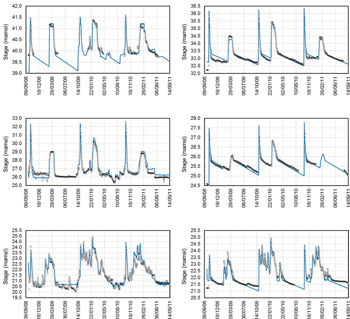
**Figure 9.16 Measured (black markers) and modelled (blue-shaded lines) stage fluctuations for the gauged locations along the Pongola River and in the pans: row-wise from top-left to bottom-right: Msenyeni Pan, Tete Pan, Lake View (River), MandlaNkuzi Pan, Ndumo (River) and Nyamithi Pan.**
