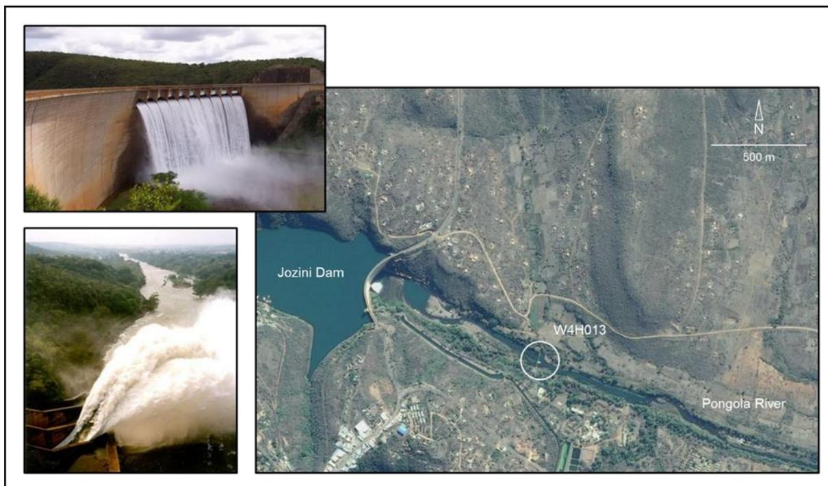
**Figure 9.3** Satellite image (GE, July 2013) of the Jozini Dam Wall and downstream Pongola River. The inset photographs show (top) the dam spilling and (bottom, after *Basson et al. 2006*) a managed release. The position of the downstream gauging station (W4H013) is indicated.
