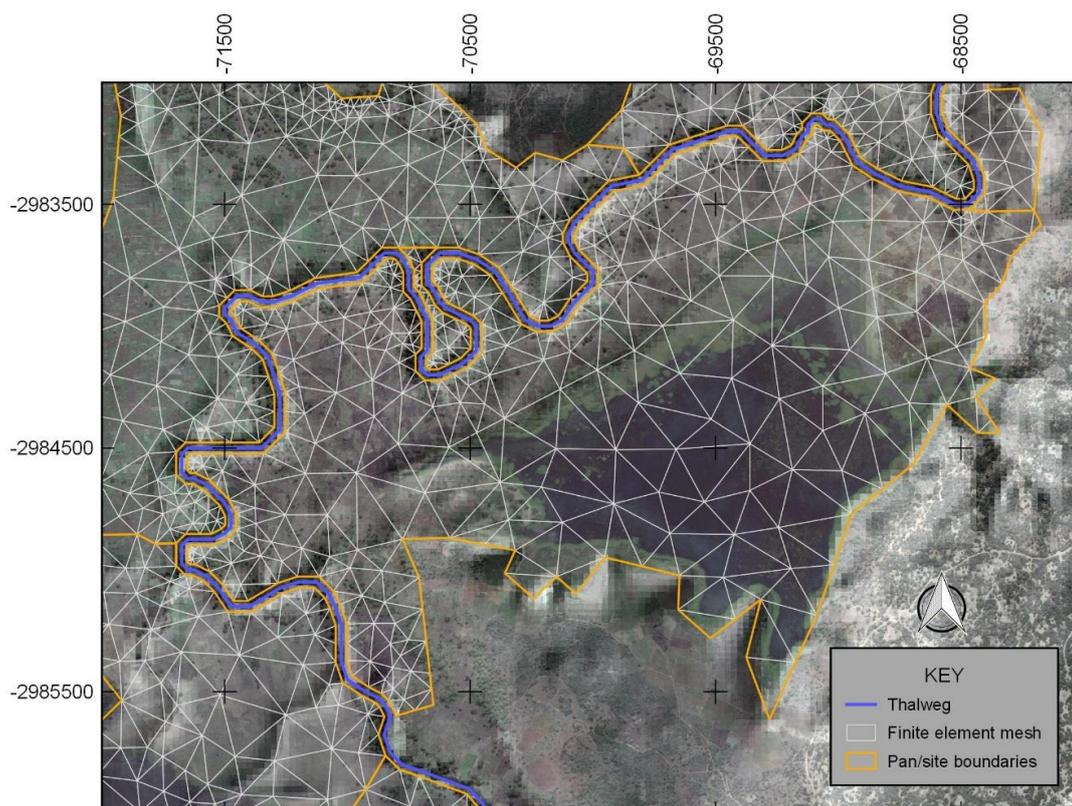
**Figure 9.15** Finite element mesh for a section of the Pongola Floodplain shown superimposed on a satellite image (GE, August 2013) which is draped over the national 25 m DEM. The projected Coordinate Reference System (CRS) is Hartebeeshoek94/Lo33.
