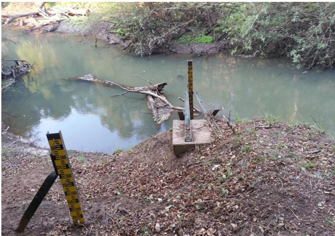
**Figure 9.11** Water level gauge W4H009 (refer to Figure 9.13) in an active channel at Ndumo Game Reserve (M. Kempen, undated).
