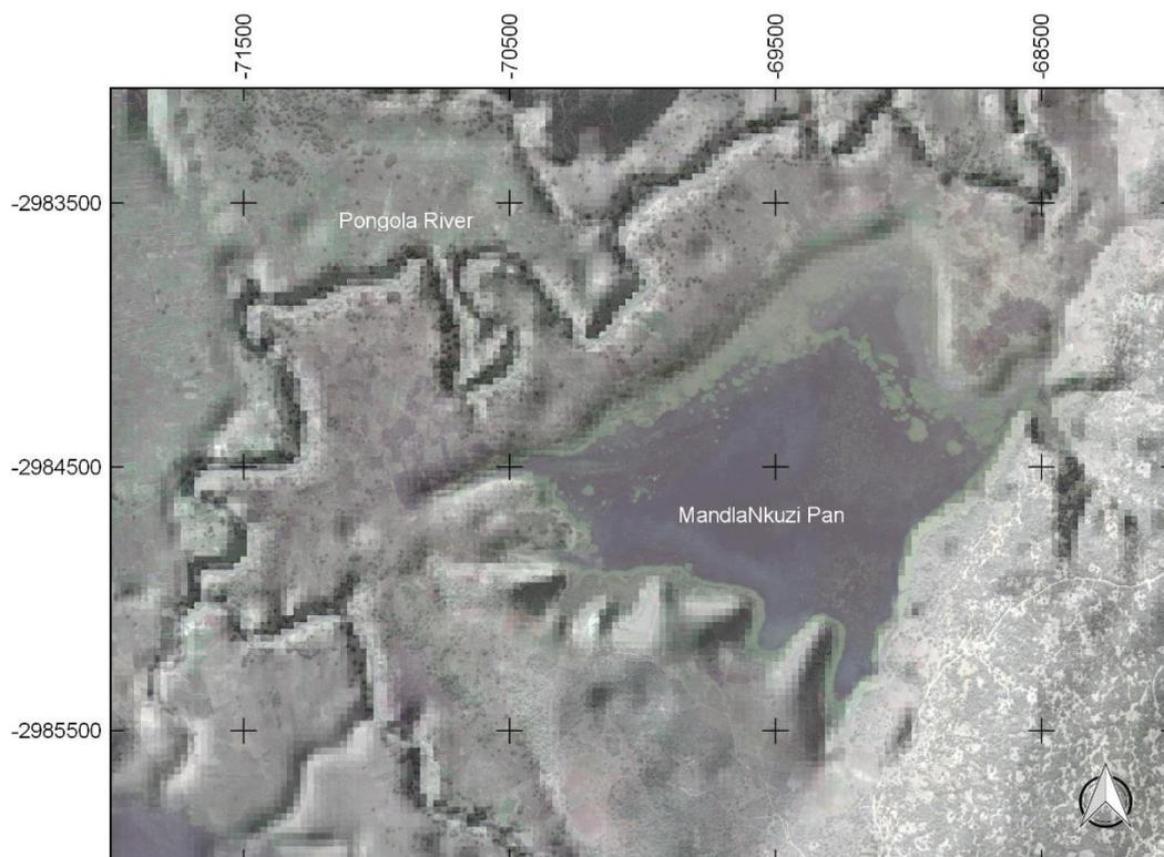
**Figure 9.5** Satellite image (GE, August 2013) of the Pongola Floodplain draped over the national 25 m DEM, showing the well-defined meandering active channel (c. 15 m wide at this location), the MandlaNkuzi Pan and patchwork of agricultural fields in the floodplain (between the pan and channel). For spatial perspectives, refer to Figure 9.12 and Figure 9.13.
