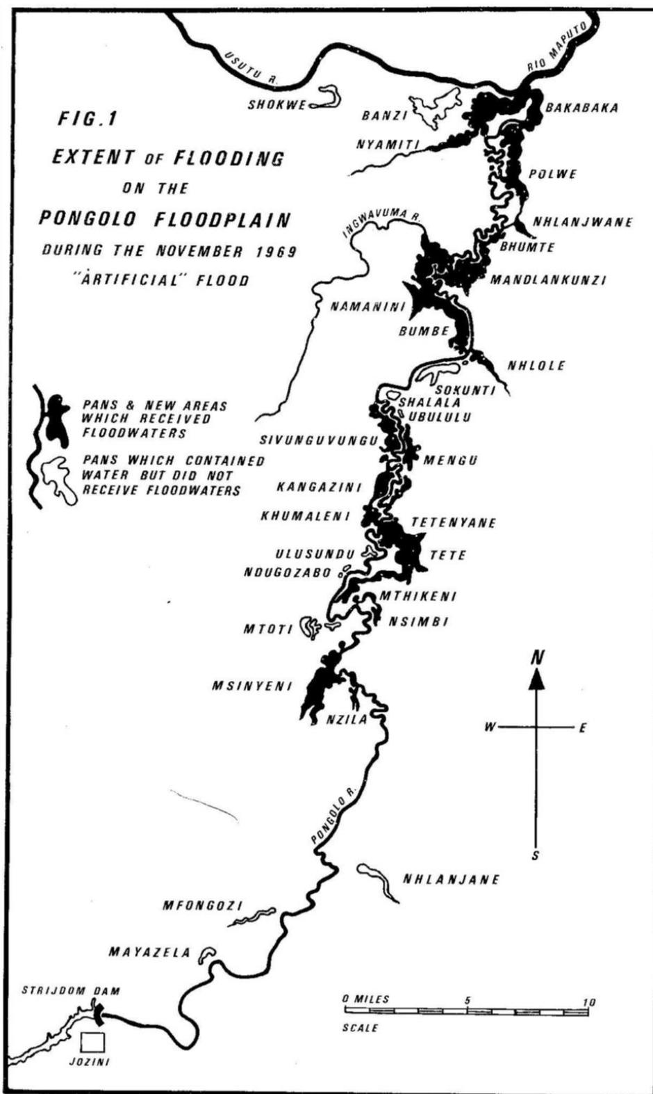
**Figure 9.2 Major Pongola Pans<sup>15</sup> and the extent of flooding in response to a release from Jozini Dam in November 1969 (after Coke, 1970)**
